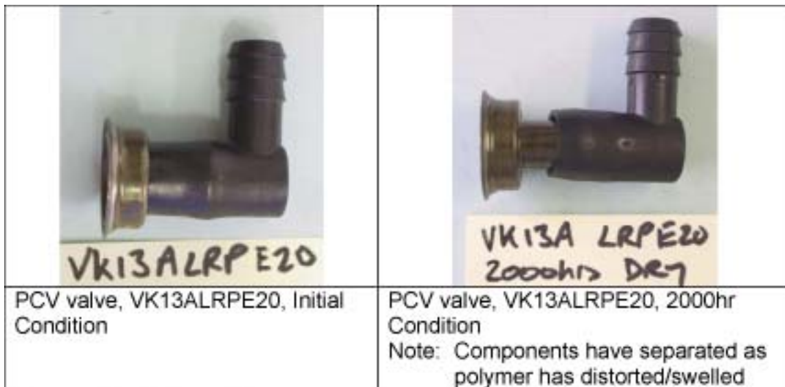
Fig. 3.12. PCV valve after immersion in E20. Source: Ref. 5.
