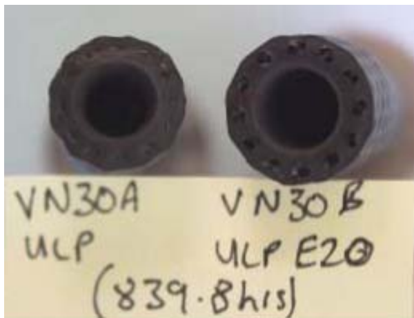
Fig. 3.10. Fuel injection return hose shown on the right after immersion in E20. Source: Ref. 4.
