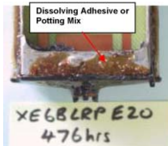
Fig. 3.11. Fuel pressure sensor after immersion in E20. Source: Ref. 4.
