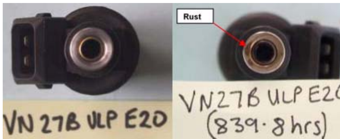
Fig. 3.6. Fuel injector showing rust after immersion in E20. Source: Ref. 4.
