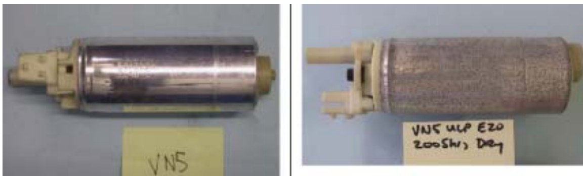
Fig. 3.8. Pitted fuel pump shown on the right after immersion in E20. Source: Ref. 5.
