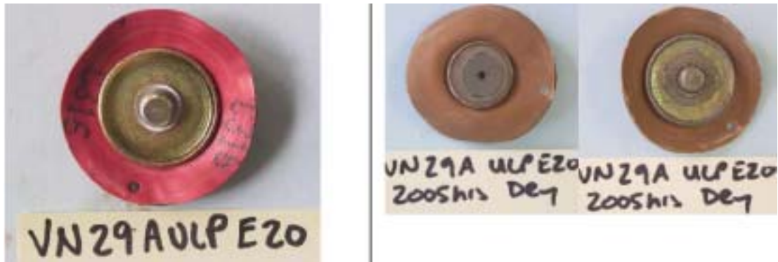
Fig. 3.7. Fuel pressure regulator diaphragm showing rust and discoloration after immersion in E20. Source: Ref. 5.
