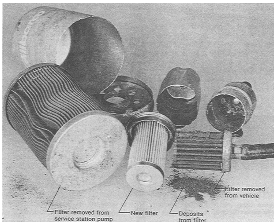
Fig. 3.4. Fuel filters plugged from introduction of ethanol blends. Source: Ref. 1.
