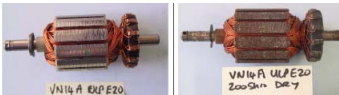
Fig. 3.5. Fuel pump commutator showing rust and tarnish after immersion in E20. Source: Ref. 5.
