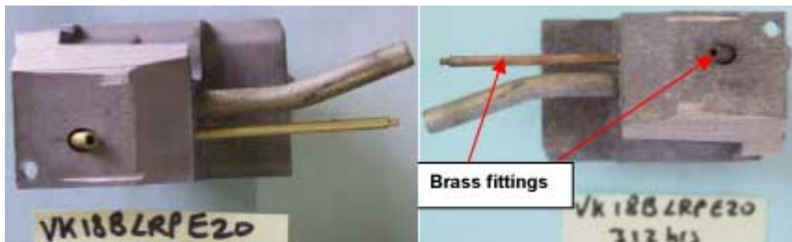
Fig. 3.9. Pitted carburetor housing and corroded brass fittings shown on the right after immersion in E20. Source: Ref. 4.
