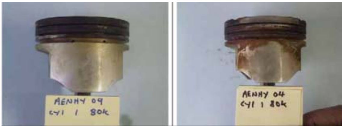
Fig. 3.13. Piston deposit after 50,000 miles of operation on gasoline (left) and E20 (right). Source: Ref. 6.
