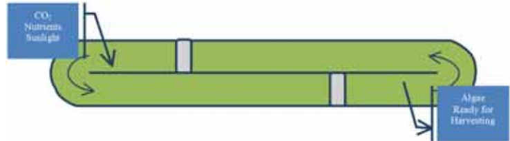
Figure 2 Single algae raceway with two motorized paddles
