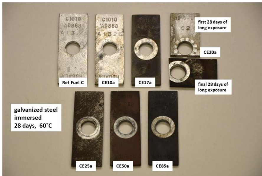
Fig. 46. Post-exposure appearance of the galvanized steel specimens. For the CE20a exposure, portions of two different specimens are included from the planned interval testing. 12
