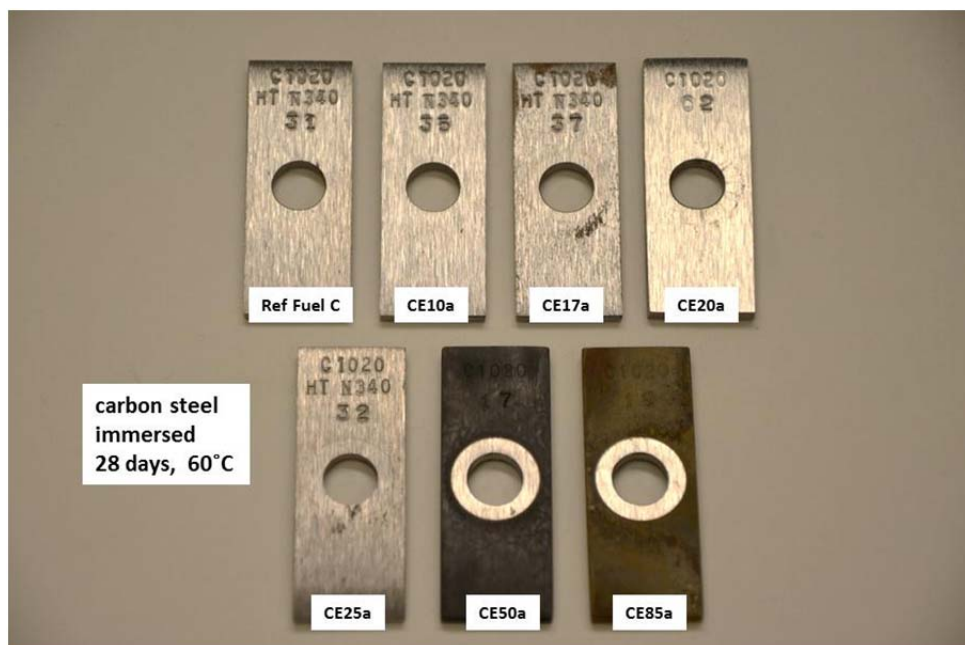
Fig. 44. Post-exposure appearance of the carbon steel specimens.
