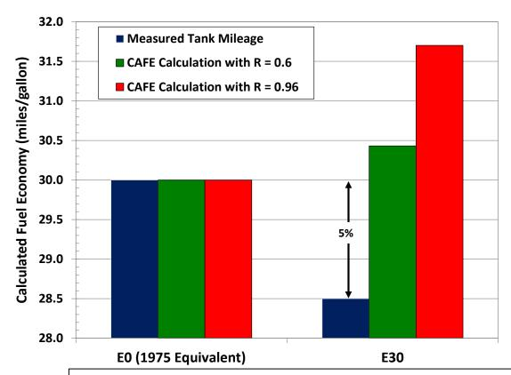
Example for illustrative purposes. Arbitrary 30 mpg base E0 FE, arbitrary assumption that equivalent vehicle with future high compression, downspeeded engine achieves 28.5 mpg.
