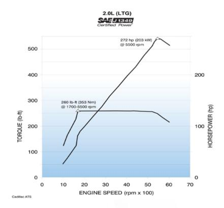
New LTG engine is excellent candidate for downspeeding/downsizing enabled with high-octane fuels
